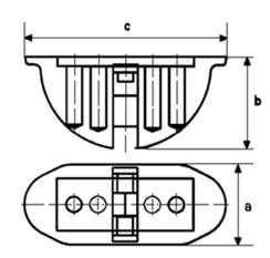
Forming device for the spread anchor lifting system, installation occurs through a fixing plate. The former provides a void for insertion of a ring clutch.
