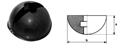
Forming device for the spherical head anchor, complete with fixing plate. The former provides a void for insertion of a lifting shackle.
