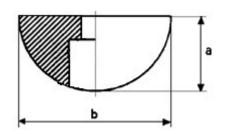
Forming device for the spherical double head anchor, complete with fixing plate. The former provides a void for insertion of a lifting shackle.
