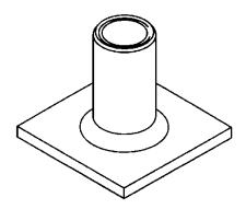
Plate end sockets comprise a threaded socket with a flat plate welded to its base Reinforcement bars can be positioned directly on the flat steel, transmitting the tensile forces safely onto the concrete The reinforcement plate may be welded or tied to the plate.
